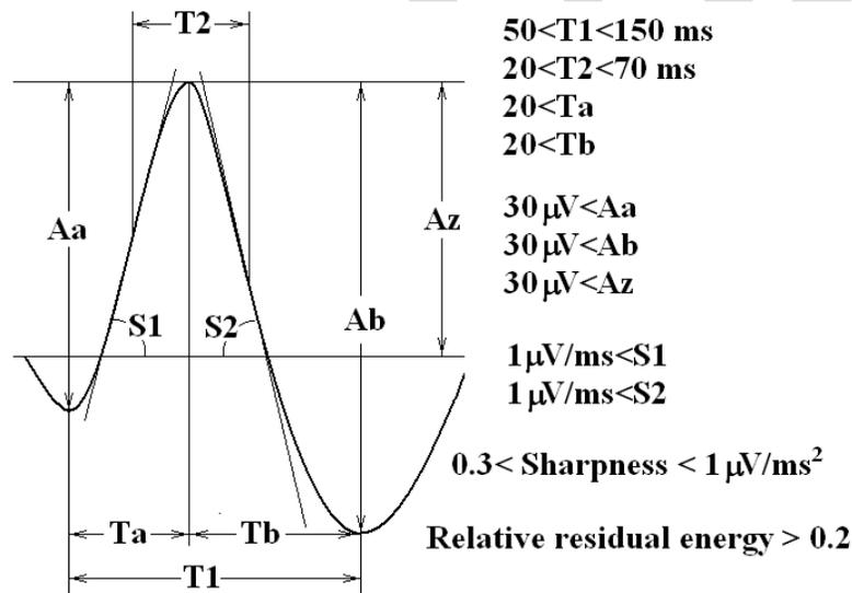
The relative residual energy for dipole approximation of the detected spike is chosen less than 0.2.
